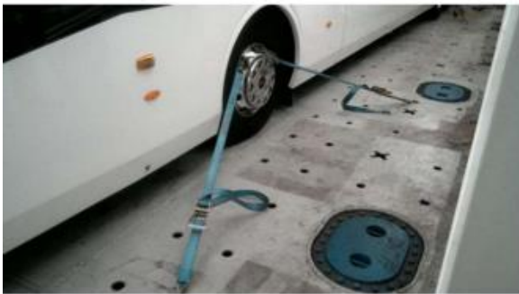
C-5 H&H cargo stowing on decks and proper stowage on rolltrailer (Mafi).
